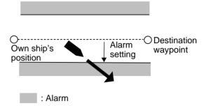
Figure 9-7 How the XTE alarm works
